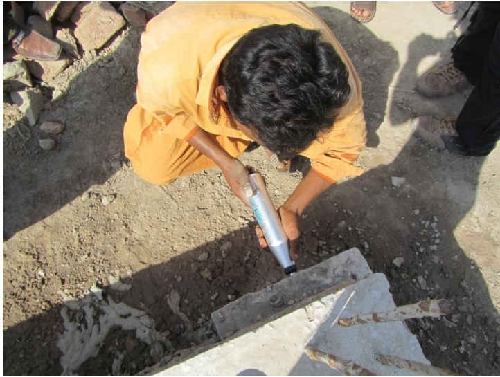
Beneficiary Training for the use of the Schimidhammer for concrete strength testing.
