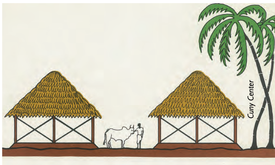
Shelter design elevation showing cross-bracing
