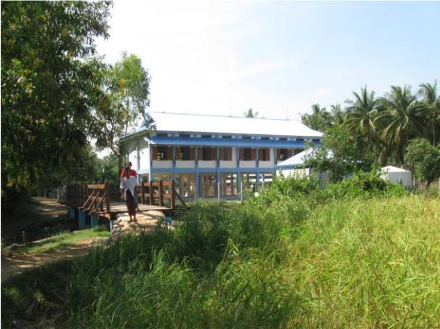
**Light, air, sun, dust, glare, reflection, humidity:** Classrooms have good fresh air circulation to avoid heat and excessive humidity. To ensure adequate daylight, more than 20% of the classroom floor area is window area. Classrooms are sufficiently shaded from direct sunlight, glare (direct light) and reflection (indirect light).
