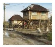
Houses on stilts in flood-prone areas at the foot of Mt. Pinatubo, Philippines. A simple mean to cope with flood damage.
