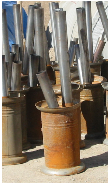
photograph: left and centre UNICEF stoves for distribution: Maslack camp 12//03/02 right: IDP amended UNICEFstove. Maslack camp 18//03/02
