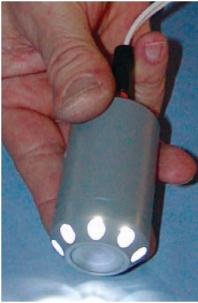
Figure 19: A CCTV borehole camera
