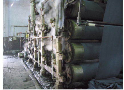
(left) The canvas is rolled through a bath of rot proofer / dye. (right) The canvas is dried on heated drums, Lahore, march 2002
