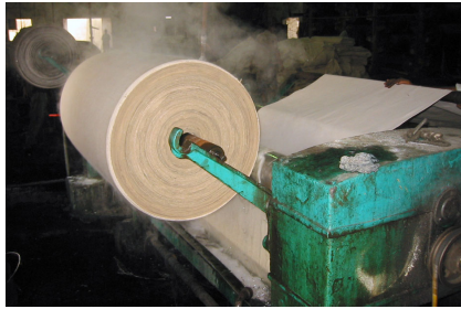
(left) The canvas is rolled through a bath of rot proofer / dye. (right) The canvas is dried on heated drums, Lahore, march 2002
