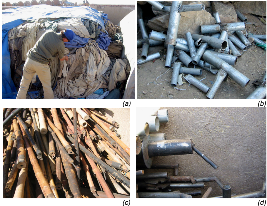
damaged tents in camp management compound, Maslack, Herat (a) damaged canvas, (b) damaged joints, (c) damaged bamboo poles, (d) damaged end spikes for steel poles
